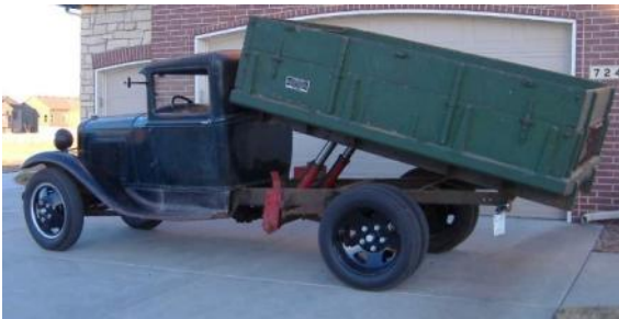
Hydraulic lift was installed by the 2nd owner
