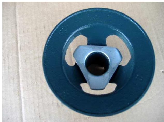
Large washer, fabricated by Grady to clear the spokes on the pulley.
