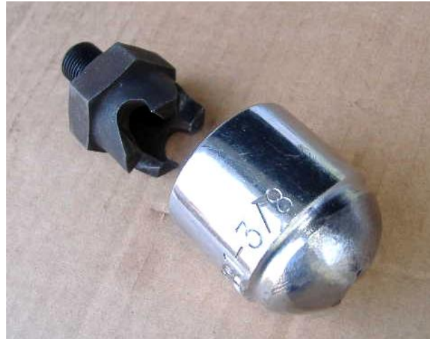
Scott Guinty had this socket with the bulk ground off the end so it will access the pulley and ratchet nut.
